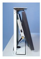
A compact gas cylinder at the back of the monitor mount allows a tilt adjustment of 10° to minimize glare and create a preferred viewing angle. A locking device secures the LCD against tampering and theft.
